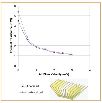
Figure 3. Effect of Anodizing on Thermal Resistance of an ATS-440-C1-R0 Heat Sink
