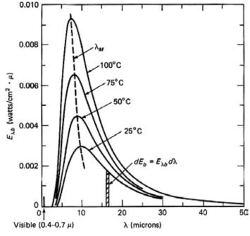
at all wavelengths, Figure 1.Low Temperature Spectral Distribution of Emissive Power without reflecting, [2].
