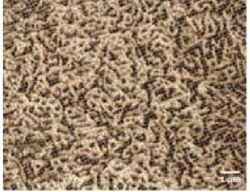
Figure 2. Ion Beam Textured Surfaces [3].
