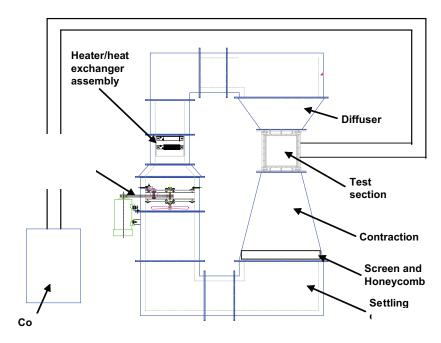
Figure 1. Schematic of an ATS Closed Loop Wind Tunnel.
