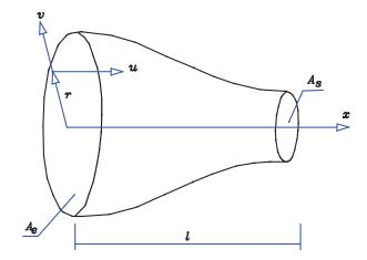
Figure 2.-Schematic of an Axisymmetric Contraction [4].
