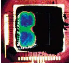
Figure 1. Component with Hot Spot as Demonstrated by Liquid Crystal Thermography. Hot spot temperatures can be 5 to 30K higher than other areas of the microprocessor, and their temperature differences can surpass 100K for optoelectronic components [1].
