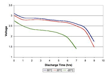
Figure 2. Discharging Performance of a Sample Lithium-Ion Battery Pack as a Function of Temperature [3].
