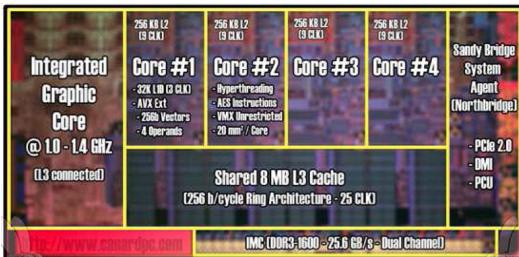
Figure 1. A Modern Intel Processor Showing the Integration of CPU, GPU, Cache and Northbridge Controller [1].
