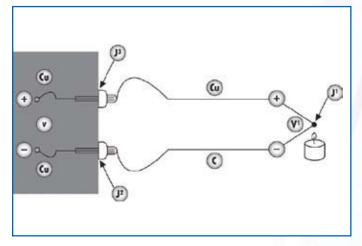
Figue 1. Measuring junction voltage with a DMV [1].
