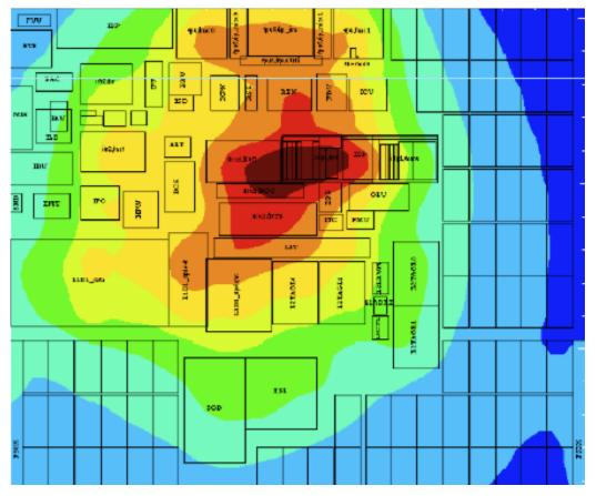
Figure 1. Color Contour Map Depicting Thermal Gradients on a Microprocessor [1].
