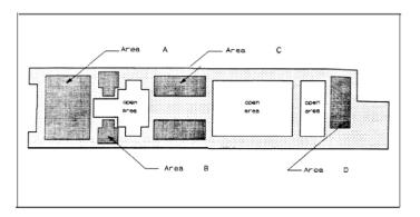
Figure 1. Schematic of a Board with a Localized Area of Heat Dissipation [1].
