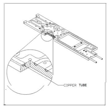
Figure 3. Schematic of the Press-Fit Tube Cold Plate Design [1].
