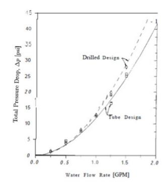
Figure 4. Total Pressure Drop of the Drilled Design and the Tube Design as a Function of the Volumetric Flow Rate [1].
