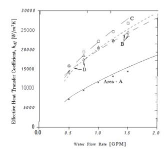
Figure 6. Effective Heat Transfer Coefficient of the Drilled Hole Design as a Function of Flow Rate for Different Regions on the Plate [1].
