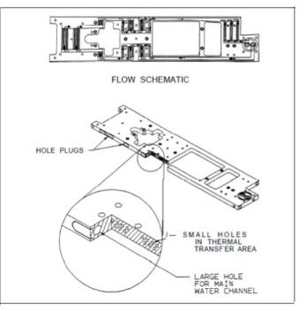
Figure 2. Schematic of the Drilled Hole Cold Plate Design [1].
