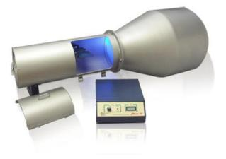
Figure 1: Servo Controlled Wind Tunnel and Control Console [1]
