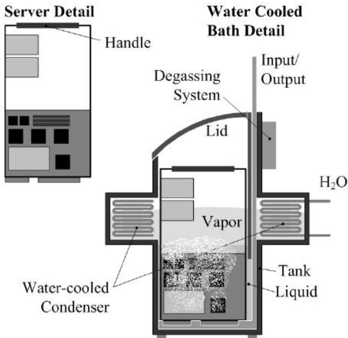
Figure 3. Passive Two-phase Immersion Cooling System from 3M [2]
