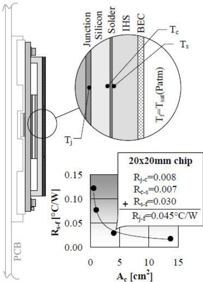
Figure 4. Application of Boiling Enhanced Coating (BEC) [2]
