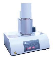
Figure 2. The Linseis LFA 1000 Laser Flash Instrument for Determining Thermal Diffusivity, Conductivity and Specific Heat Values [3].
