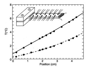
Figure 3. Data Obtained by Measuring the In-Plane Thermal Conductivity, k of a Sample of Printed Wiring Board with Many Vias [2].
