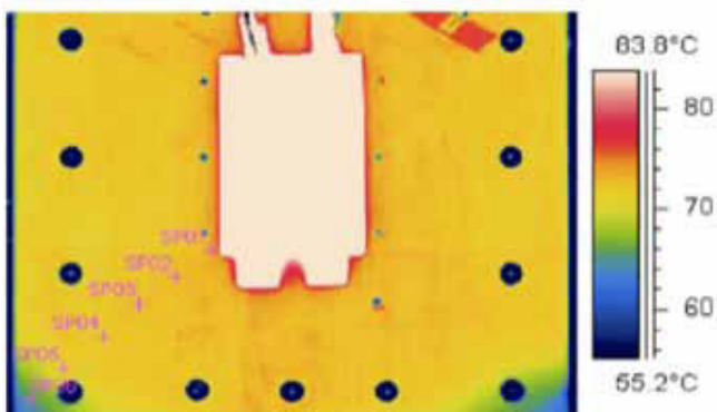
Figure 4. Effects of Wick Thermal Conductivity on Junction Temperature [5]
