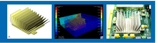
Figure 2. SolidWorks Images of the ATS-725 maxiFLOW<sup>™</sup> Heat Sink Along with its CFD Simulation and Prototype.
