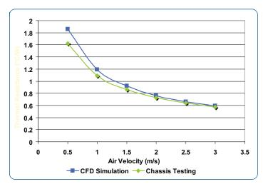
Figure 5. The Results of CFD Simulations and Chassis Testing of the ATS 725 maxiFLOWTM Heat Sink. GE Fanuc Recommends and Airflow of at least 275 LFM if a Passive Heat Sink is Used
