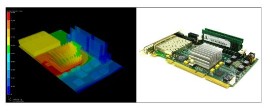
Figure 4. CFD Simulation of the GE Fanuc Intelligent Platform's WANic Packet Processor PCI Card with the ATS-725 maxiFLOW™ Heat Sink Installed, Along Side a Sample Card.
